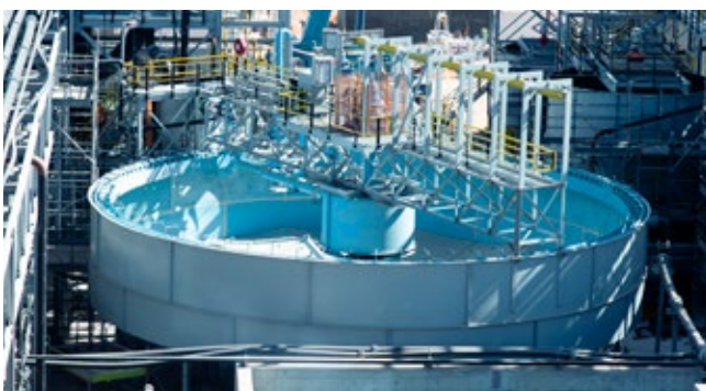
High-rate bolted thickener for iron ore, 18 m in diameter
