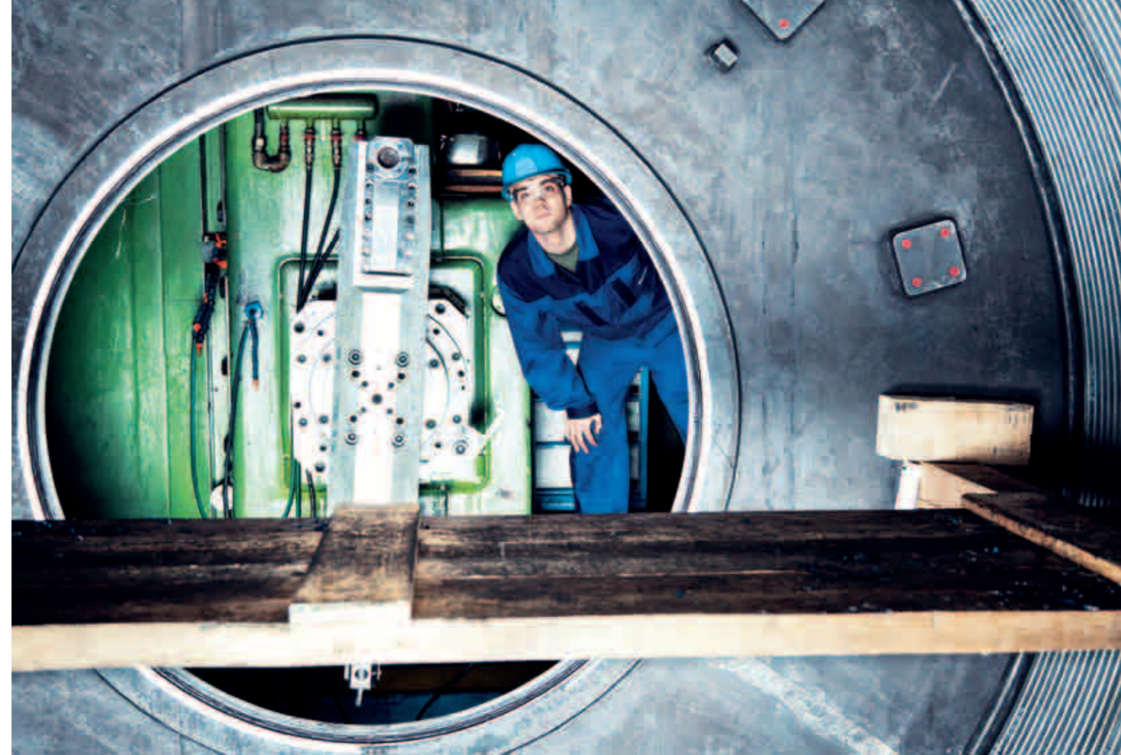
▲ Steel Yankee cylinder being machined on a horizontal boring mill.
