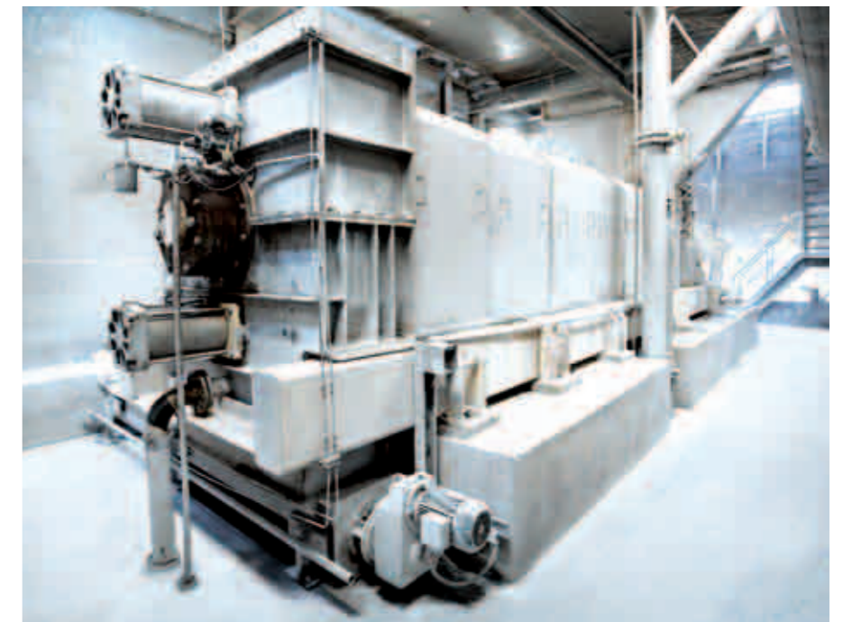
The SCS 1008 screw press was rebuilt and upgraded over the weekend with the ANDRITZ Mobile OSR service. ▼
