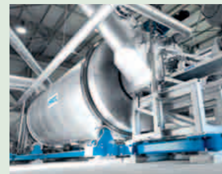
◀ The torrefaction pilot plant in Frohnleiten, Austria is based on ANDRITZ’s ACB (Accelerated Carbonized Biomass) process. It uses an indirectly heated drum reactor (shown here) that is designed for up to 50,000 t/a production.
