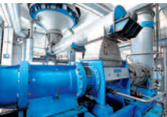
▲ MSD Impressafiner in the existing Yinhe plant is the first key stage in the ANDRITZ P-RC APMP process.
