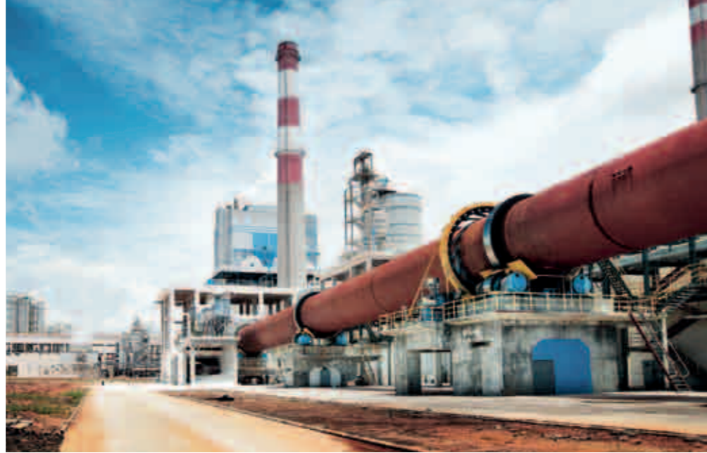
▲ The White Liquor Plant from ANDRITZ uses the latest LimeGreen green liquor filtration systems. ANDRITZ also delivered the kiln, white liquor oxidation, and LimeWhite white liquor filtration equipment.
