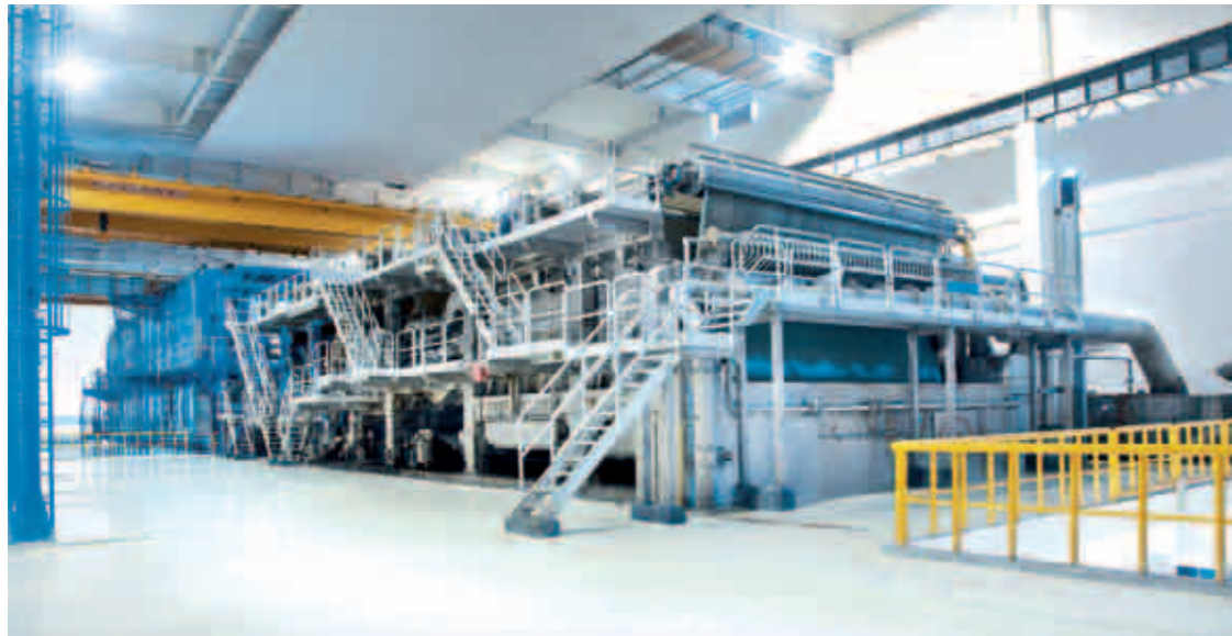
◀ Top left: The ANDRITZ airborne pulp dryer produces the dried pulp sheets.
