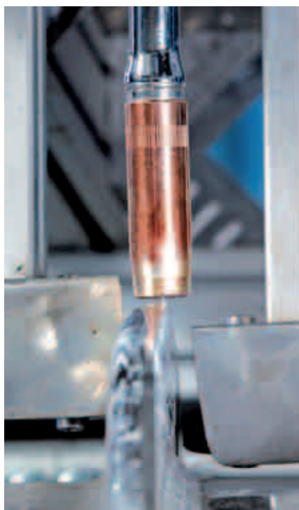
Close-up of the screw flight welding tip on the Mobile OSR unit. ▼
