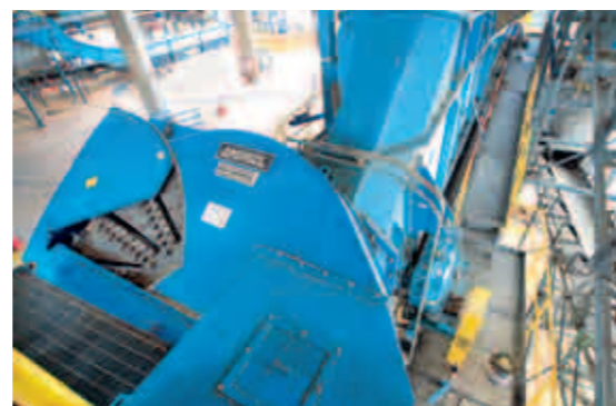
▲ The debarking drums (above left) were dimensioned to handle both long and short logs. Two HHQ-Chipper lines (one shown above) deliver uniform eucalyptus chips to the digester.
