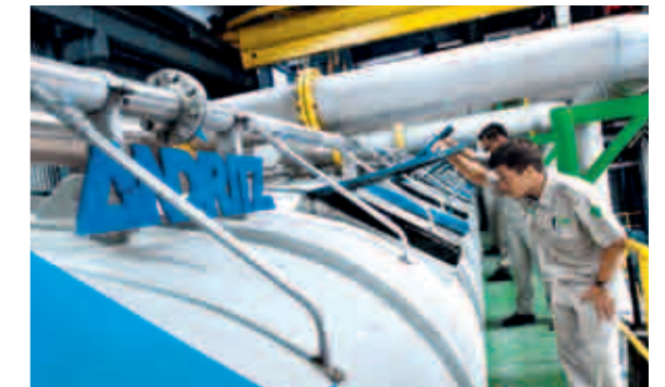
▲ The pulp's brightness boost begins with effective ink removal in SelectaFlot deinking.
