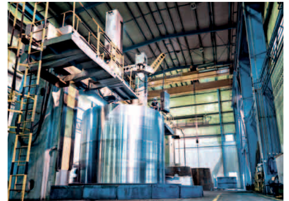
▲ Turning a Steel Yankee cylinder at ANDRITZ Kft.
