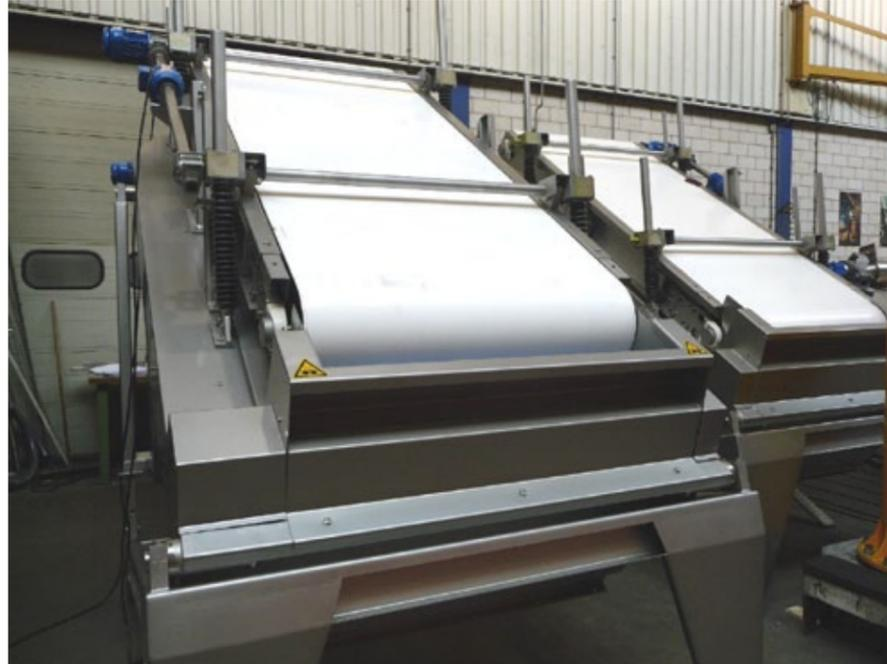
More than 300 Brush 'n Belt dry peel removers have been installed since ANDRITZ Gouda started development of this machine in 1975. Most of the machines are integrated into industrial steam peeling lines that may include an ANDRITZ Gouda Sepa-Stator steam peeler, a Brush 'n Belt dry peel remover, a peel waste pump, and a post-washer. In the steam peeler, the product is subjected to intensive, but extremely short steam treatment.
